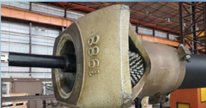
*Inserting System to 155mm Gun*
